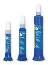
Threadlocking, for locking after mounting and sealing of hair cracks. Due to its low viscosity and high capillary effect, it penetrates into the intermediate spaces of the threads. A previous loosening of the connection is not necessary. Ideal for pre-assembled threaded joints.
