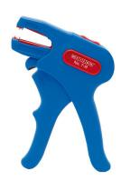
The WEICON Wire Stripper No. 7-R has a precise adjustment (5-fold ) and an optical length scale of 8 - 24mm (5/16 - 1 inch). This allows flexible round cables of 0.5 - 16.0 mm² (24 - 10 AWG) and solid round cables of 0.5 to 10 mm² (18 - 15 AWG) to be stripped. The Wire Stripper No. 7-R is also suitable for two-core, PVC-insulated flat cables of 0.75 - 1.5 mm². An easy-to-access side cutter is integrated into the tool and can be used up to a cable diameter of 3 mm. It also has exchangeable
